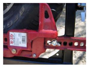
Mount Hi-Lift Jack to the lower tabs on the tire carrier using the included 1/2" carriage bolts, flat washers and wing nut.
