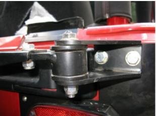
Remount the upper hinge arm to the tire carrier. Insert two of the 3/8" x 1.25" bolts with flat washers through the tub of the Jeep.
