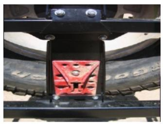
Before installing the Hi-Lift jack to the tire carrier, remove the foot pad and secure to the antenna post using a 5/16" x 1" carriage bolt through the center as shown in the photo.
