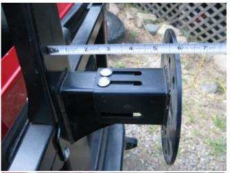
Using the measurement from the previous step, measure and adjust the wheel hub and antenna post to the right offset. The wheel hubs will secure to the antenna post using the 5/16 x 3/4 carriage bolt, flat washers and lock nuts.
