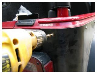
Remove the upper hinge arm from the carrier. Pull back the carpet from the inside of the tub where you will be drilling.
