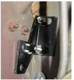
Install the latch bracket backing plate inside the fenderwell as shown using two of the supplied 3/8" bolts, washers, and lock nuts.
