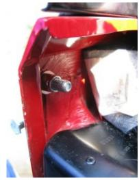
Insert three of the 3/8" x 1.25" bolts with flat washers. Tighten the upper bolt with a flat washer and lock nut.
