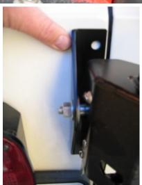
Take the latch pin bracket (with the latch pin installed) and lock it into the latch mounted to the tire carrier. Push the tire carrier against the body and mark the centers of the 3 holes.
