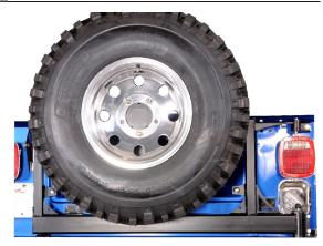
Portions of the tire carrier, and corresponding rear bumper come with parts pre-installed by Hanson Offroad. The rear spindle bumper (JRR4102-P) will have the latch pin, scuff block, spacer plates and rubber stopper installed. The tire carrier (CTC2-P) will have the spring loaded locking pin assembled on the pivot side of the carrier and the upper latch installed on the opposite side. The upper tub bracket will have the latch pin installed as well.
