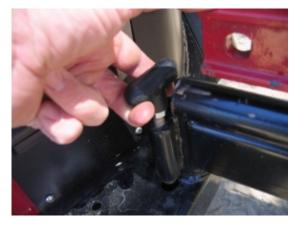
Place Hi-Lift along the tire carrier to allow for easy access to the dead-man pivot handle as shown.
