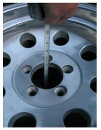
Using the spare tire, set the rim down on a flat surface and measure to the backside of the rim. Subtract 3/4" and use this measurement in the next step.
