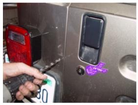
Drill through the tub with a 1/4" pilot bit. Once all three holes have been started, open them all up using a 7/16" drill bit.
