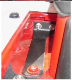
Remove the outside roll cage bolt. Install the upper hinge backing plate as shown using two of the 3/8" bolts and supplied flat washer and lock nuts.
