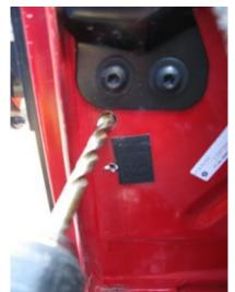
Drill through the piloted holes with a 7/16" drill bit as shown in the photo
