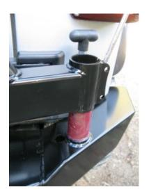
Lube the spindle on the bumper with a water resistant auto or marine grease.
