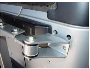
Bolt the upper hinge arm to the tire carrier using two of the 3/8" x 1.25" bolts and corresponding flat washers and lock nuts.
